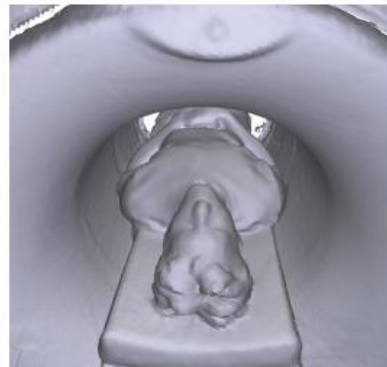
Fig. 2. Kinect surface created using the Point Cloud Library opensource implementation [2] of the KinectFusion algorithm [3].
