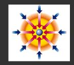
Shocks forming as the fuel compresses converge in the compressed fuel and raise the fuel to 100 million degrees Kelvin
