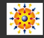
Higher density material heats and blows off (ablation), rest of fuel is compressed to 1000 x solid density via rocket action
