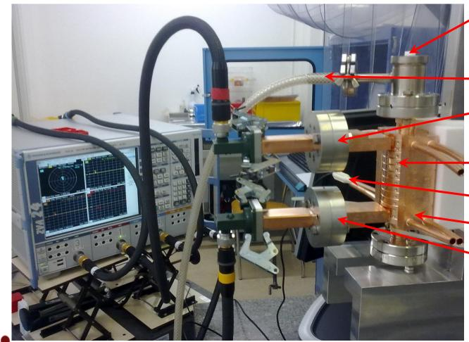
centring V guiding the wire for beadpull measurements nitrogen supply input (chosen and marked) tuning pins (4 per cell) temperature sensor cooling block output (marked)
