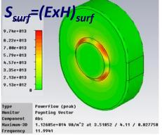
• Peak electric and magnetic fields of the dipole mode are located 90 degrees from each other on the iris
