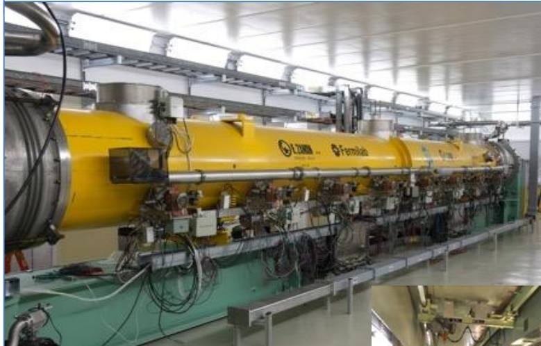
Cryomodule test at Fermilab reached < 31.5 > MV/m, exceeding ILC specification
