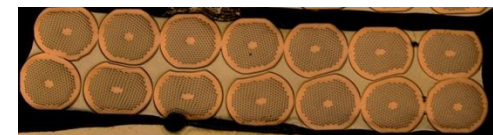
1 mm, 192 tubes PIT from Bruker EAS
