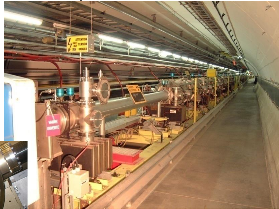
20m of SPS septa move together-LSS2
