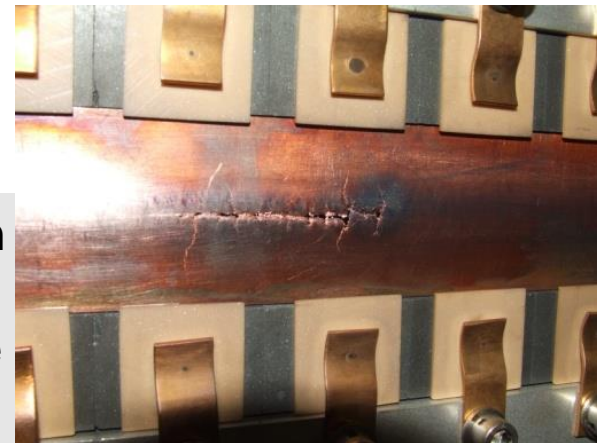
Fatigue failure on the mid plane of the septum blade of PSB BISMH
