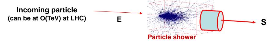
**Calorimetry: basic mechanism**
