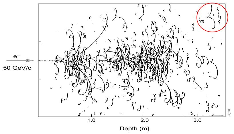
Big European Bubble Chamber filled with Ne: $H_2 = 70\%:30\%$ , 3T Field, L=3.5 m,  $X_0 \approx 34$  cm, 50 GeV incident electron
