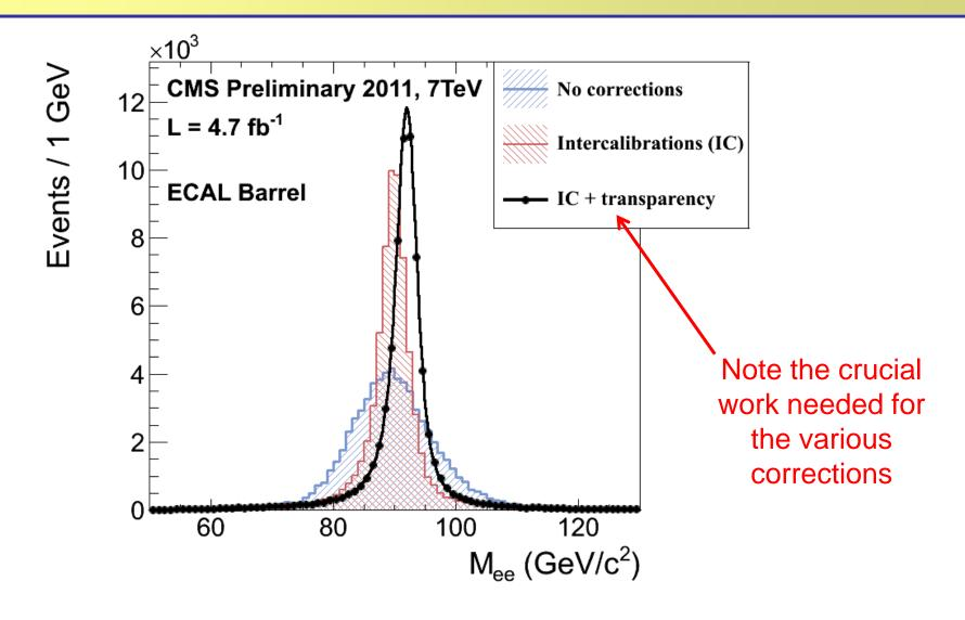
Instrumental resolution of 1.01 GeV from Z -> ee decays in the CMS ECAL Barrel
