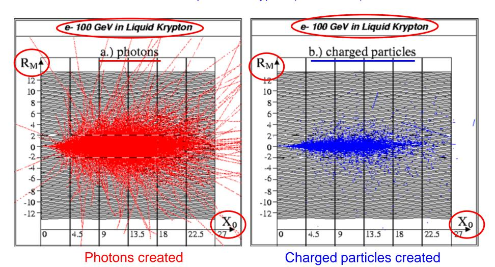
GEANT simulation: 100 GeV electron shower in the NA48 liquid Krypton calorimeter
