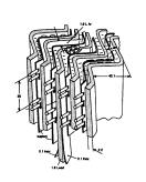
Corrugated stainless steel clad Pb absorber sheets,1-2 mm thick
