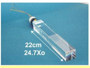
CMS Endcap crystal, tapered, 3x3 cm<sup>2</sup> at rear Vacuum Photo Triode readout, gain ~ 8
