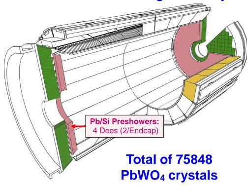
**Barrel:** 36 Supermodules (18 per half-barrel) **61200 Crystals** (34 types) – total mass 67.4 t
