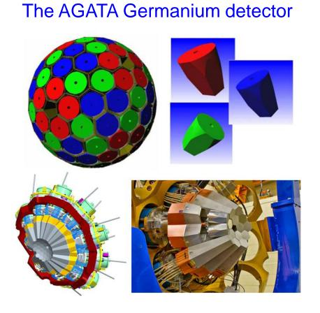
Experiment with excited nucleii from a target 1382 keV line width 4.8 keV (fwhm) Resolution 0.15%
