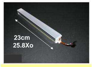
CMS Barrel crystal, tapered ~2.6x2.6 cm<sup>2</sup> at rear Avalanche Photo Diode readout, gain = 50
