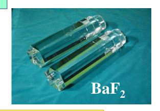
Crystals are basic components of electromagnetic calorimeters aiming at precision
