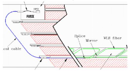
Light produced in the scintillators is transported through optical fibres to Hybrid Photo Diode (HPD) detectors
