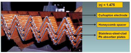
Accordion geometry minimises dead zones Liquid argon intrinsically radiation hard Readout board allows fine segmentation (azimuth, rapidity, longitudinal)
