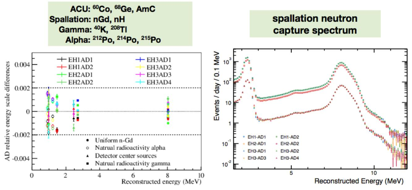
Less than 0.2% variation in reconstructed energy between detectors
