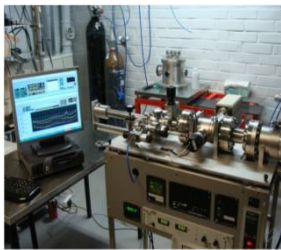
General view and scheme of TDS apparatus
