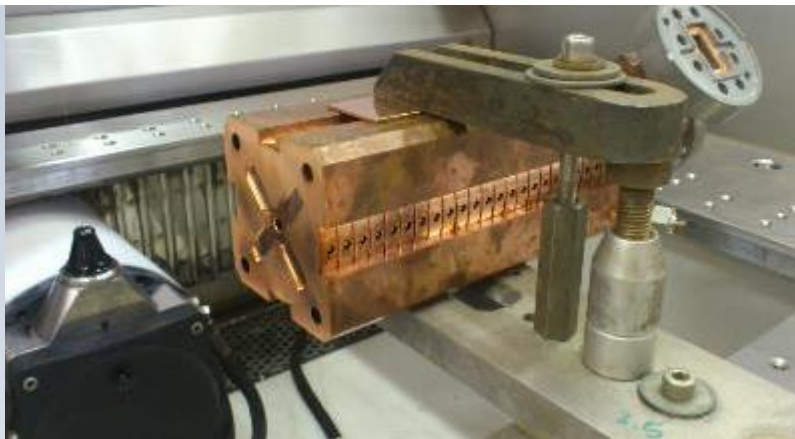
EDM wire cutting machine at CERN workshop:
