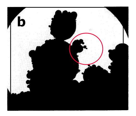
One logical explanation of the circled effect is that the thermodynamic drive changes several times as the protrusion is growing.
