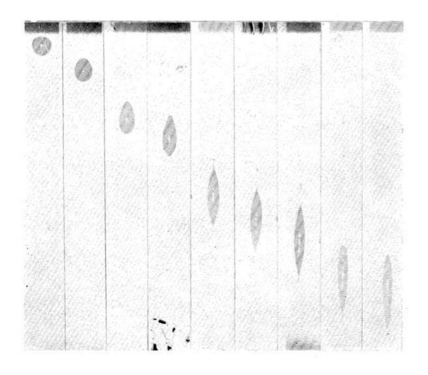
Droplet falling in electric field: Courtesy: Macky, 1931.
