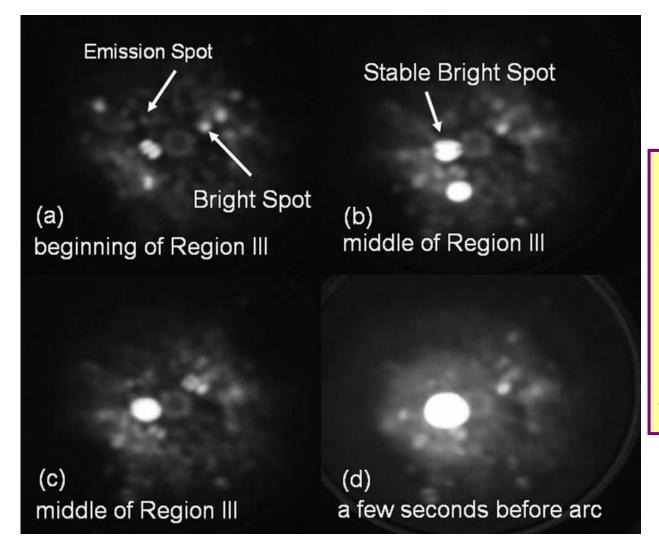
This sequence shows unambiguously that, with cold metal field electron emitters, arc initiation is preceded by nanoprotrusion growth on top of the field electron emitter.
