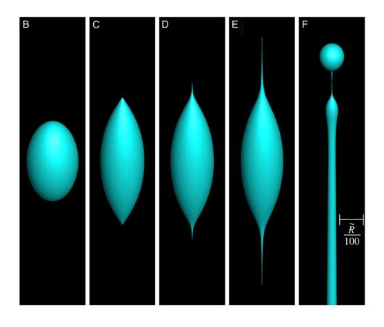
Simulation of water droplet in electric field: Courtesy: Collins et al., 2013
