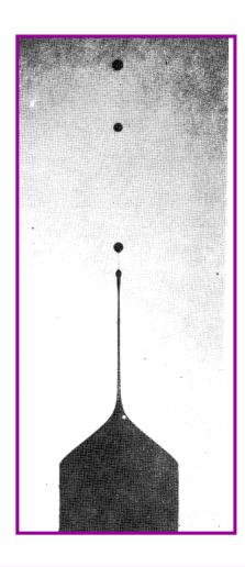
It seems clear that negative hydrostatic pressure inside the drop is drawing liquid into it
