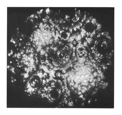
At high temperature, even a tungsten field ion emitters will "slip" under the influence of the field stresses due to high electric fields. Courtesy, Southworth et al.]
