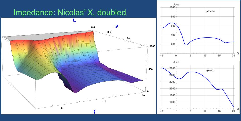
Stabilizing octupole current versus gain and chromaticity for HL LHC  $E = 7 \text{TeV}, \quad N = 2.2 \cdot 10^{11} \text{ p/b}, \quad \tau_{\text{sep}} = 25 \text{ ns}, \quad \varepsilon_{\text{n}} = 2.5 \,\mu\text{m}, \quad \sigma_{\text{H}} = 7.5 \text{ cm}.$
