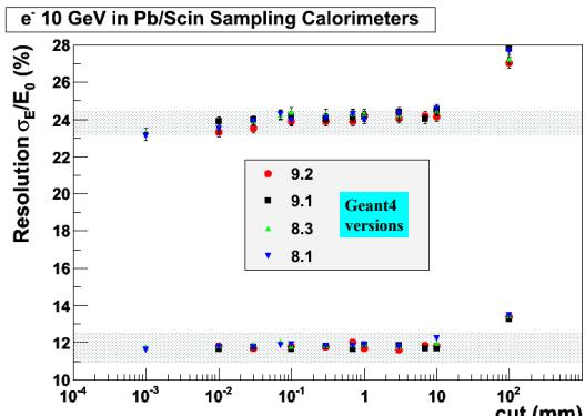
Energy resolution of sampling calorimeter as a function of the production thresholds (cut in range).
