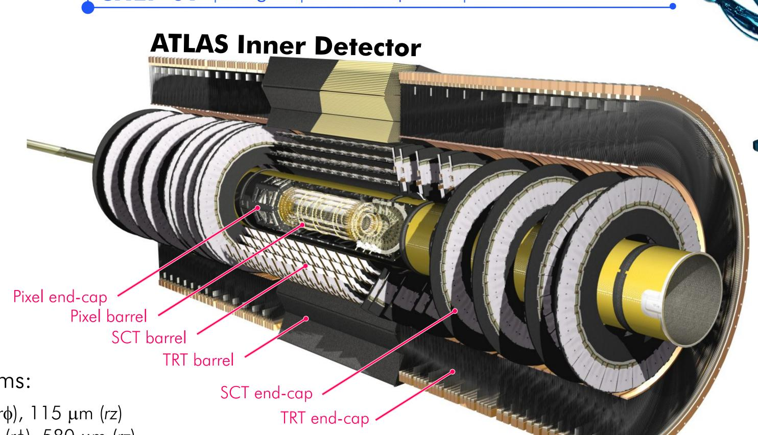
The ATLAS Inner Detector consists of three detector systems:
