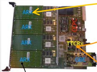
→ The TELL1 read-out board receives the analogue front-end signals from the VELO. The main tasks of this off-detector electronics acquisition board are data synchronization, buffering and zero suppression. The zero suppression (TELL1 processing) procedure, that runs after the digitization, consists of several algorithms implemented within FPGA processors. This allows to suppress the noise in the system and reconstruct clusters. Each board processes data coming from one sensor (2048 channels).
