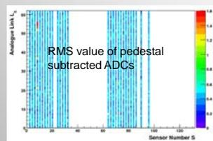
The main output stream of the emulator. The emulated ZS bank is identical to the one produced by the TELL1 board for the BIT PERFECT Emulation
