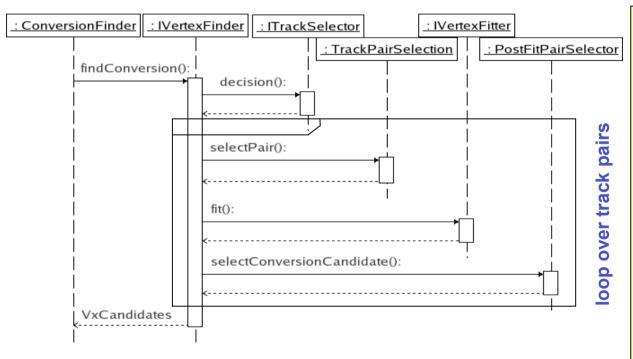
The ConversionFinder analyses a container of (electron) tracks and reconstructs conversion vertices using a dedicated *ConversionVertexFinder*. The latter pre-selects tracks using the interfaced *TrackSelector* and finds iteratively conversion candidates: a) track pair pre-selection, b) vertex fitting,
