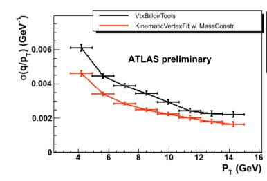
The application of the J/ $\psi$  mass constraint in J/ $\psi \rightarrow \mu^+ \mu^-$  decay leads to the improvement of resolutions on momenta of muon tracks.
