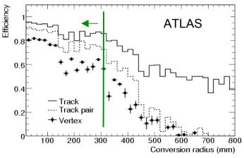
The efficiency drops at large radii because of complications in reconstructing both electrons.
