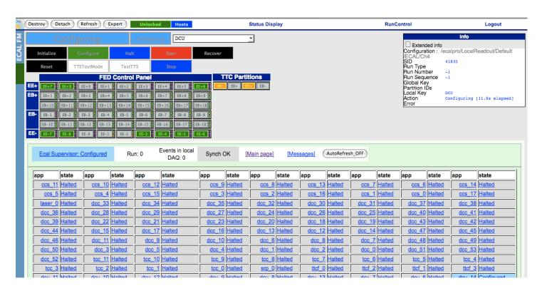
A tree of finite state machines controls the data taking operation of the experiment (Function Manager)
