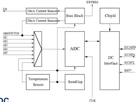
**Quantities measured with 12 bit ADC Sensitivity:**
