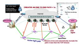
The integrated Optical Control Plane system is implemented as a distributed set of collaborating agents. It provides real-time monitoring of network topology, controls and creates on demand end to end optical paths. The distributed agents can detect partial network outages and release all allocated segments along the optical path. An alternative path might then be set up, quick enough to avoid a TCP timeout, so that the transfers can continue uninterrupted.
