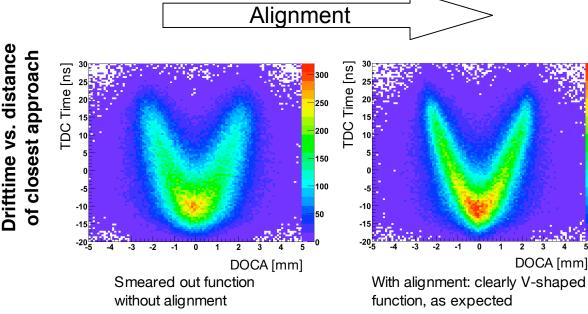
Alignment of the Outer Tracker layers and comparison of the alignment parameters with survey data. The software alignment results are in very good agreement with the survey data!
