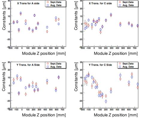
**Difference of Alignment** Constants Misalignments in X and Y direction for the TED data from August and September. A side and C side denote the left and the right halves of the VELO. The modules are in a stable position and the software gives reproducible output for the two runs. Diff. of Constants [µm] Width of the distribution: 3 µm; alignment constants obtained in August and September are in very well agreement!
