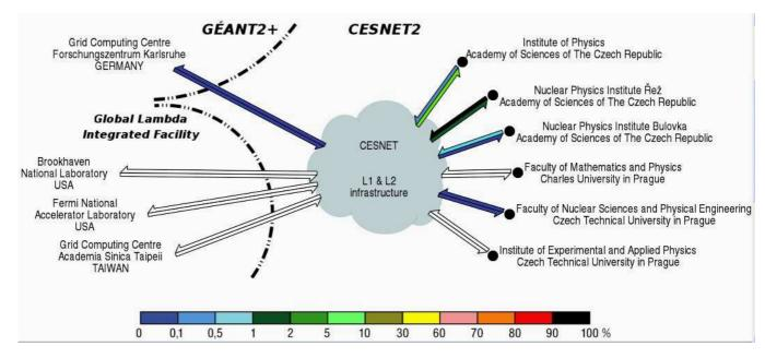
Figure 4. Topology and traffic of CESNET2, the Prague-based network facility for HEP
