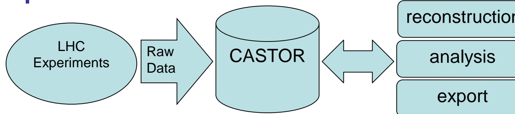
CASTOR architecture is based on the disk cache which serves to transfer data from and to the tapes. The system is able to serve thousands of requests per second, while managing millions of files.
