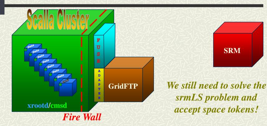
**Target Adapter: File System in User Space (FUSE)** Full POSIX file system based on XrdClient called xrootdFS Interoperates with **BeStMan** and probably StoRM
