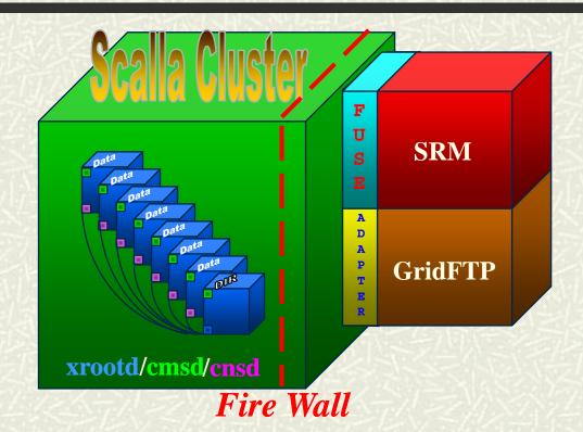
A cnsd runs on each data server node communicating to an extra xrootd server running on the redirector node
