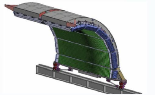
EMCal is a Pb-scintillator sampling calorimeter
