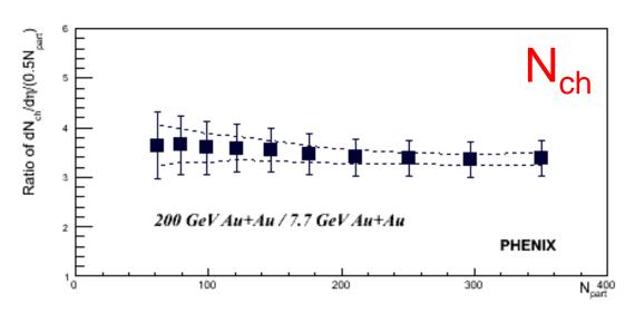
The shapes of the distributions as a function of N<sub>part</sub> do not change significantly from 200 down to 7.7 GeV.
