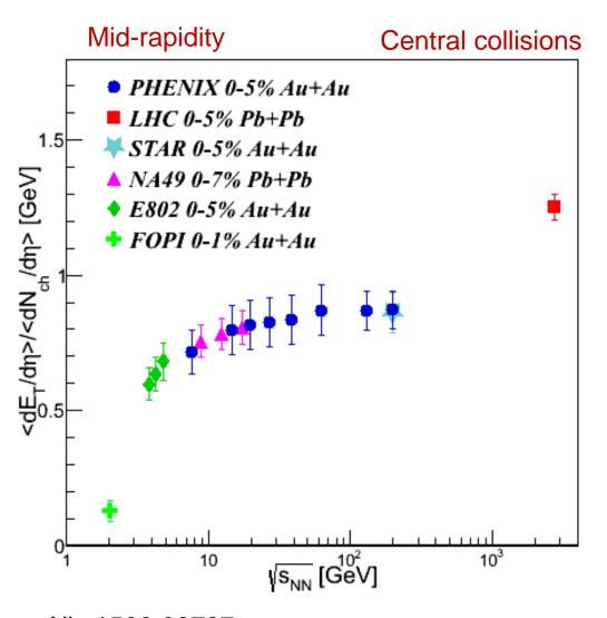
There is very little change in the transverse energy per charged particle from 7.7 GeV to 200 GeV.
