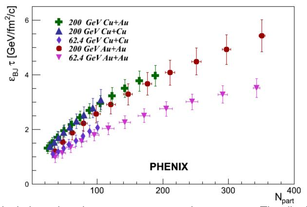
The  $\varepsilon_{bj}$  calculation takes the system geometry into account. The distributions as a function of  $N_{part}$  do not change significantly between Au+Au, Cu+Au, and Cu+Cu systems at the same collision energy. For a given collision energy (200 or 62.4 GeV), the data are independent of system size.
