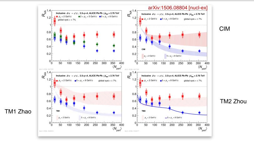
For  $N_{\text{part}}$ > 150, the suppression is larger at high- $p_{\text{T}}$  than at low- $p_{\text{T}}$
