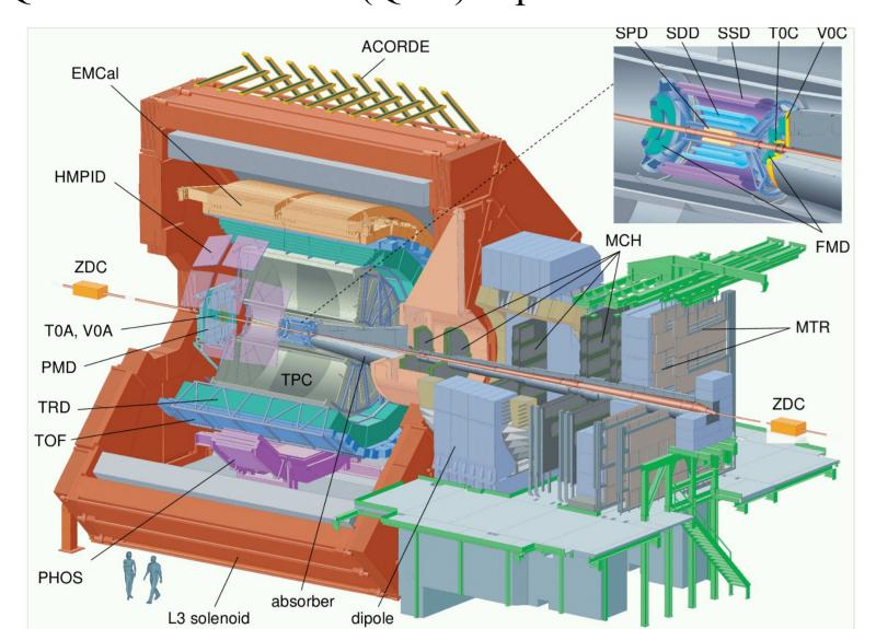
Schematic view of ALICE Detector system.
