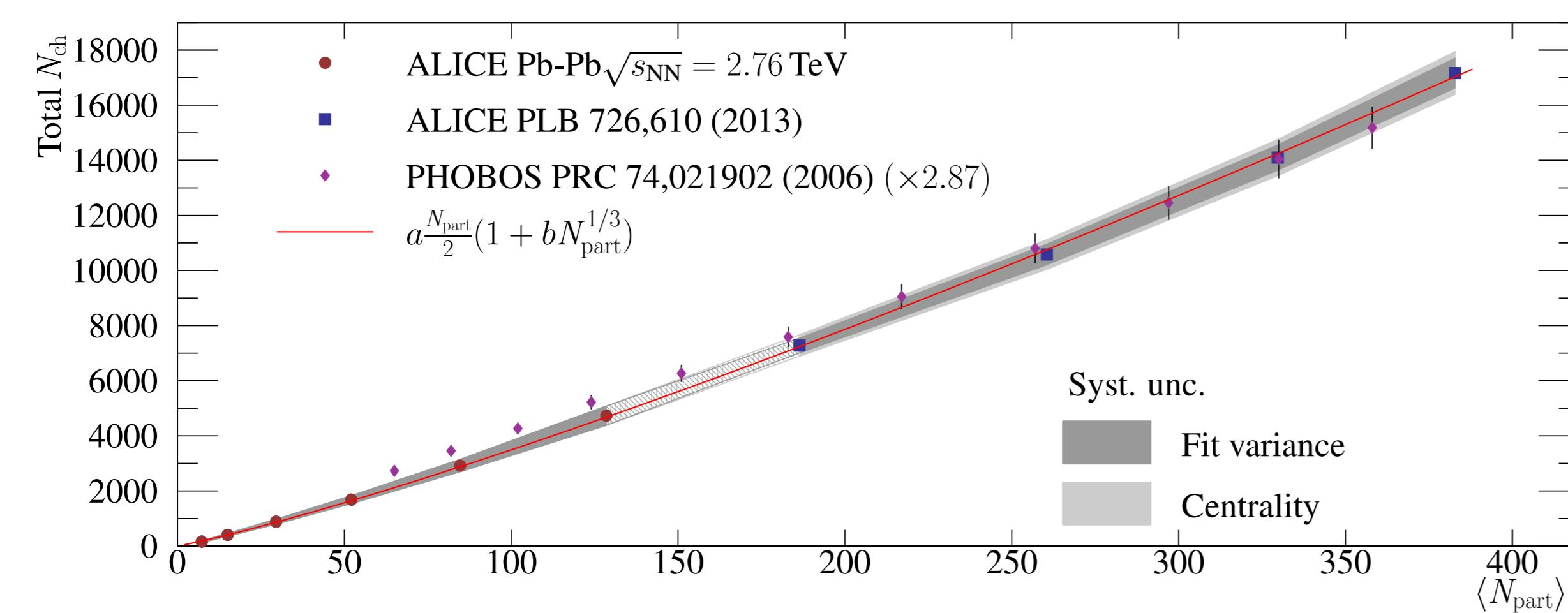
Total charged-particle production in Pb-Pb as a function of  $N_{\text{part}}$  [1]. Particle production is observed to scale near-linearly with  $N_{\text{part}}$ , similar to lower energy data [5].
