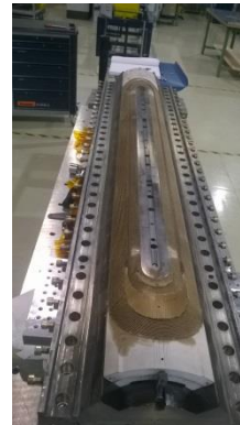
CERN coil #102 prepare for impregnation
