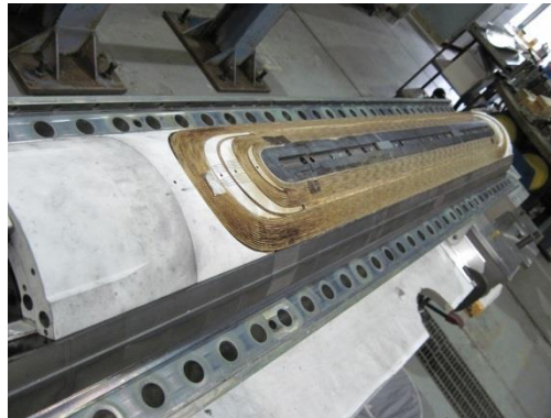
CERN coil #102 prepare for impregnation
