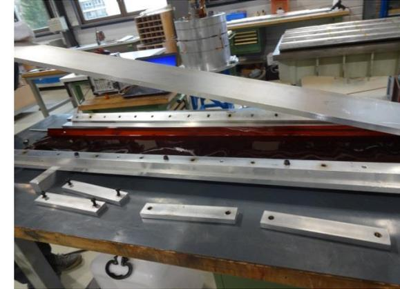
Ground insulation forming tool ready
