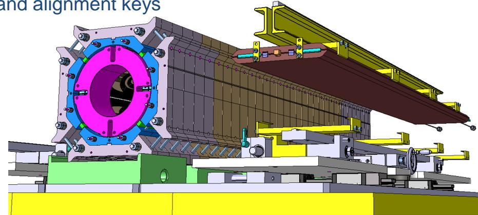
The masters are mounted and clamped to the coil-pack assembly before transportation to the insertion table
