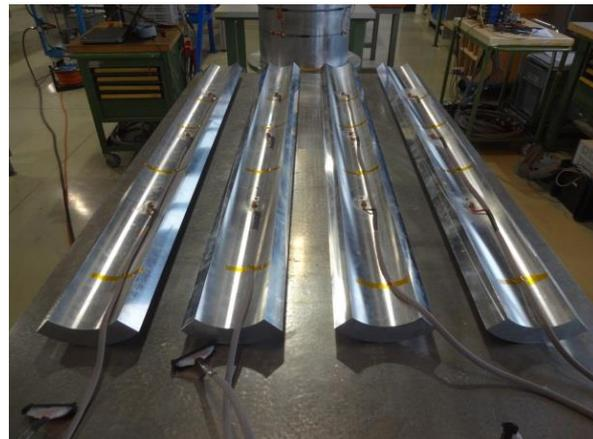
Instrumented dummy coils
