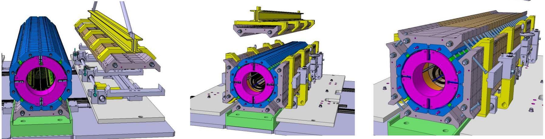
The same sequence is used to assemble and bolt the iron pads around the collars. The assembly tooling is designed to provide accurate alignment of all components during the assembly process.
