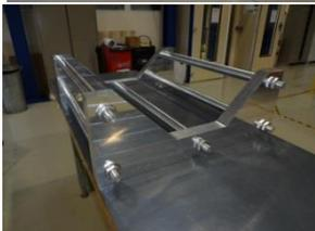
Yoke & shell support to flip from vertical to horizontal position ready.
