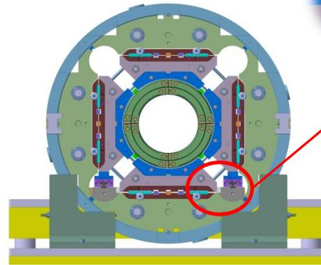
2 lateral bladders are pressurized to insert the remaining nominal keys
