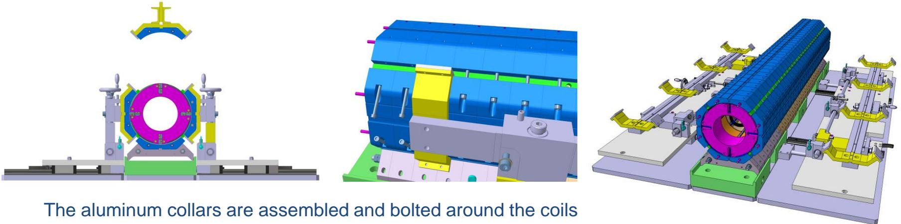
The aluminum collars are assembled and bolted around the coils
