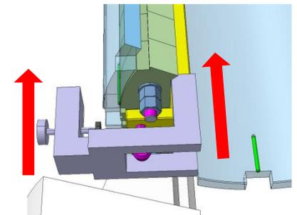
Dedicated clamping tools will be used to radially clamp the ¼ yoke in the shells
