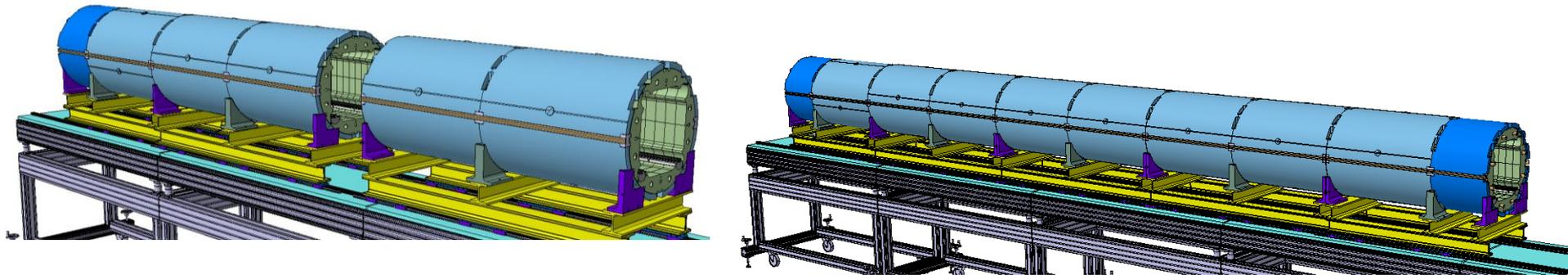
The subassembly rods will be replaced by longer ones using small hydraulic cylinders
