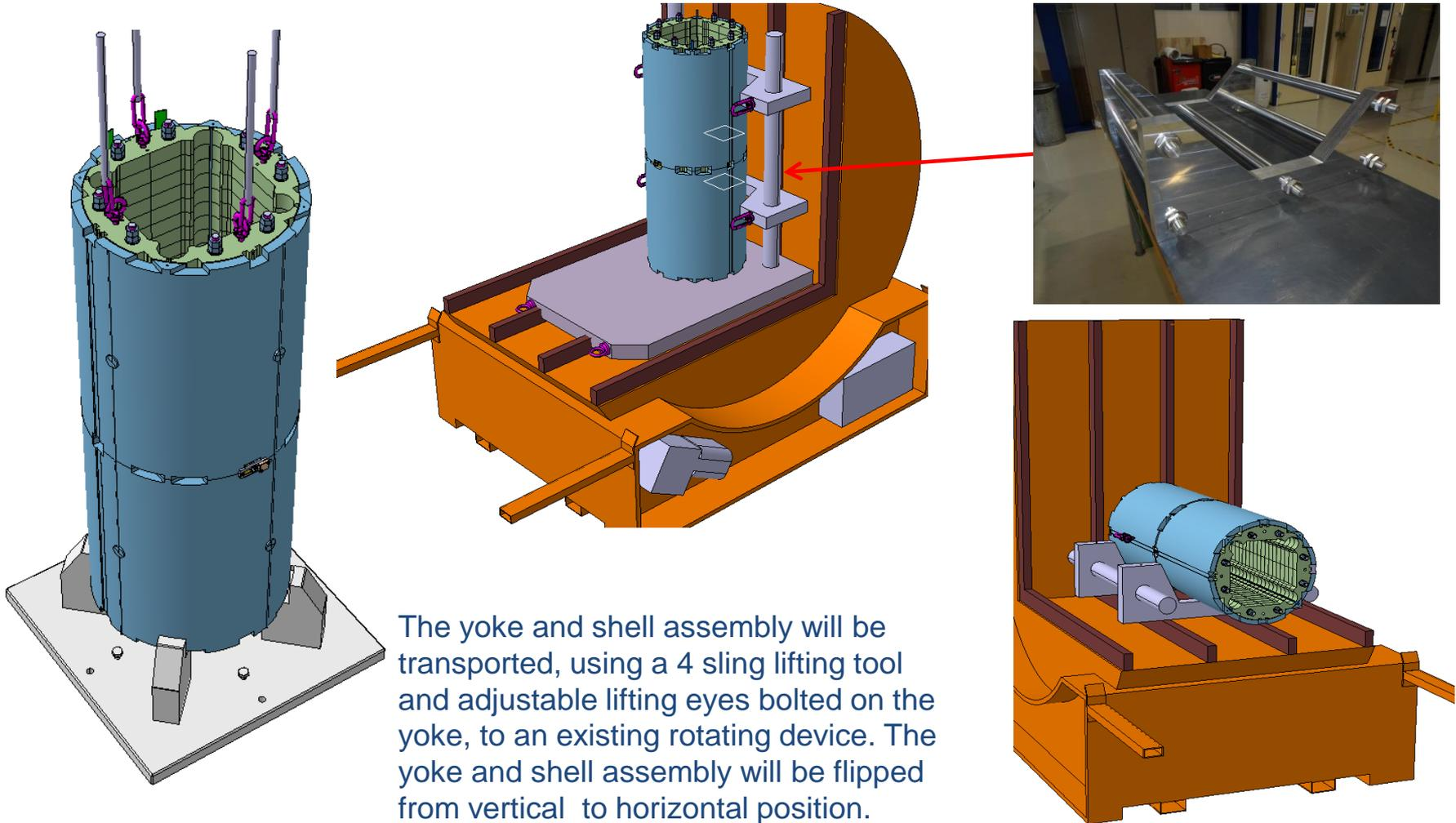
The yoke and shell assembly will be transported, using a 4 sling lifting tool and adjustable lifting eyes bolted on the yoke, to an existing rotating device. The yoke and shell assembly will be flipped from vertical to horizontal position.
