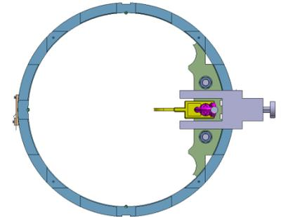
The angular alignment of the first ¼ yoke is defined by 1 long middle pin and 2 small pins located at the shell extremities
