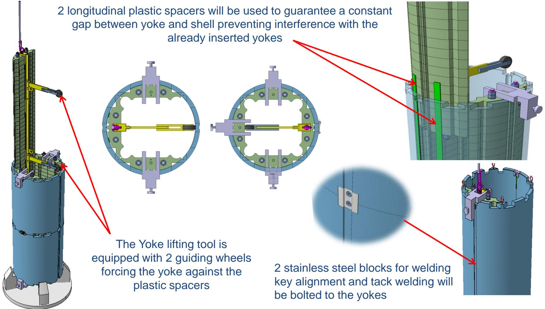
The Yoke lifting tool is equipped with 2 guiding wheels forcing the yoke against the plastic spacers
