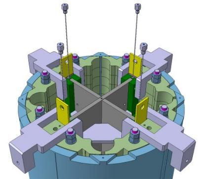
4 bladders 1549 mm \* 57 mm will be used during shell pre-loading operation.
