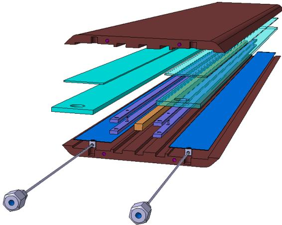
The four masters are equipped with bladders, shims and alignment keys
