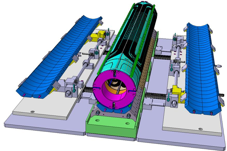
2 + 2 coils equipped with ground insulation and pole keys are positioned on top of the lower 1/4 pad and collar assembly
