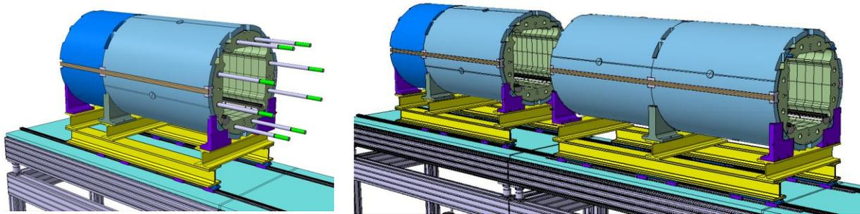
Each individual subassembly will be positioned on its support structure and assembled with the adjacent one using precision rails and linear guides.
