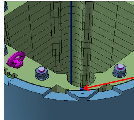
Temporary yoke keys are inserted in the yoke gaps
