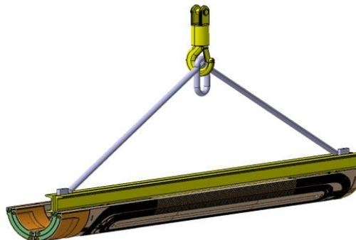
The first pair of coils to be assembled will be rotated up-side down and lifted from their inner face. The coil handling tooling is designed to manipulate the coils by pairs from inner and outer radius. The same tooling can be used to handle coils individually.
