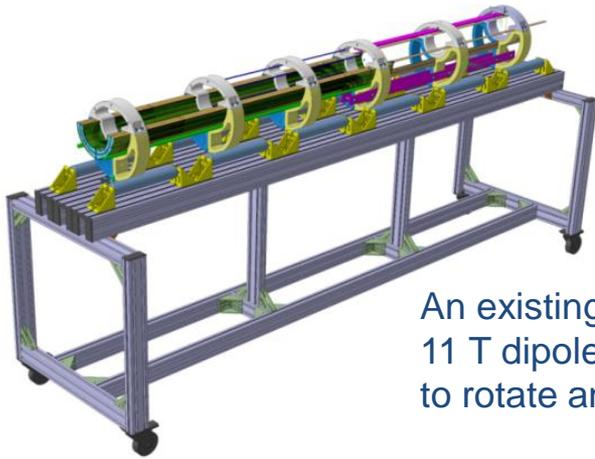
An existing assembly table used for the 11 T dipole project has been adapted to rotate and position MQXFS coils.
