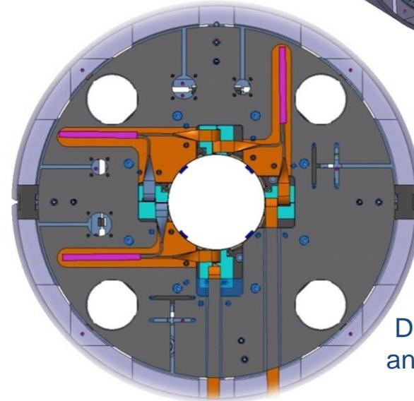
Design of the splice box and instrumentation plate in progress
