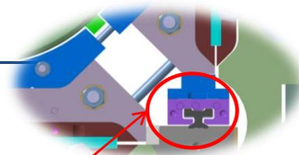
Lower bladder is pressurized. Top and bottom nominal keys are inserted.
