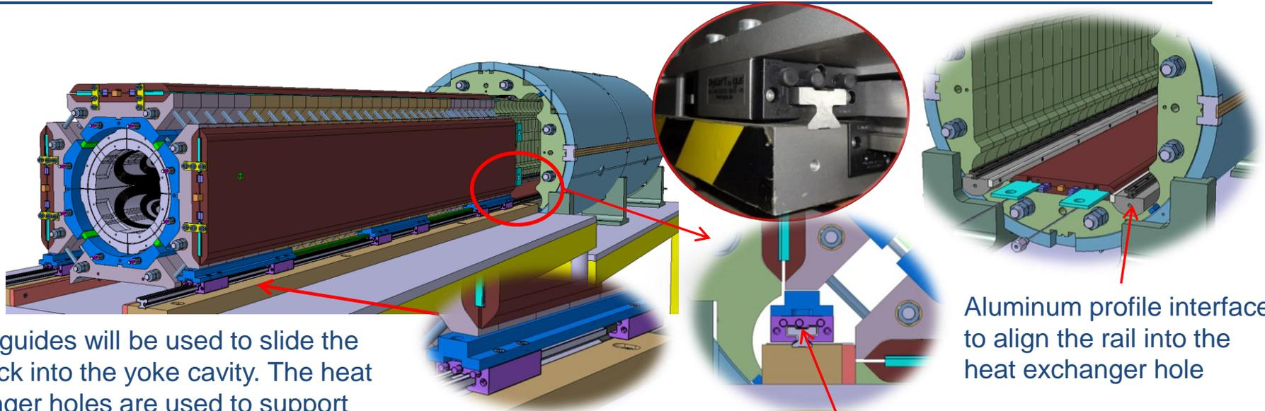
Aluminum profile interface to align the rail into the heat exchanger hole
