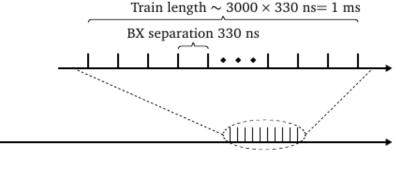
Train separation 200 ms → Repetition rate 5 Hz
