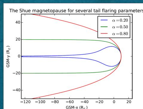
**Figure 3:** The shape of the Shue magnetopause is closed for  $\alpha < 0.5$ , opens to a finite thickness for  $\alpha = 0.5$  and open for  $\alpha > 0.5$ . The standoff distance used is  $10R_E$ .
