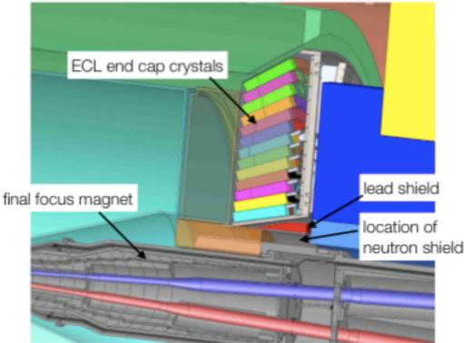
Thermal Neutron Detector System in 'BEAST II' Commissioning Detector
