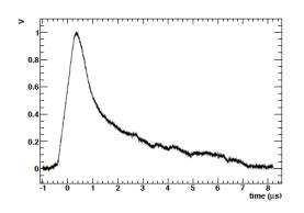
He-3 detector signal of thermal neutrons from UVic neutron
