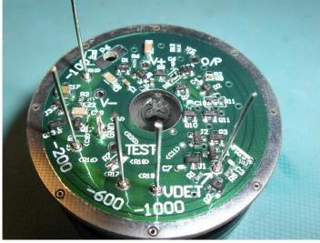
Preamplifier with HV divider
