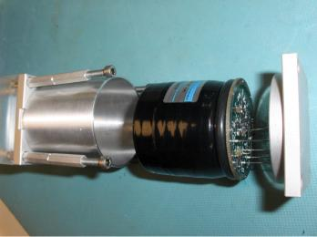
Photomultiplier mounted with preamplifier and Faraday cage
