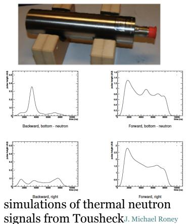
CsI(Tl) Photon Detector System in 'BEAST II' Commissioning Detector - In Phase 1 of commissioning – 2016 -Measure photon backgrounds at position of ECL from Tousheck and Beam-gas rates to validate/Correct MC simulation for projections to higher luminosities
