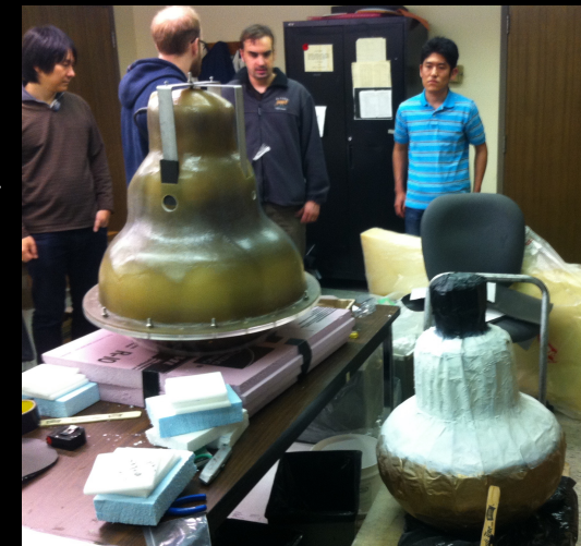
L: 20" SK PMT at TRIUMF R: papier mâché mockup
