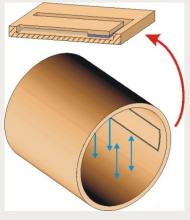
Resonator Prototype at SFU (Q ~ 300)
