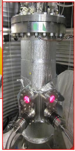
PICO-60 Pressure vessel inside the water tank at Snolab
