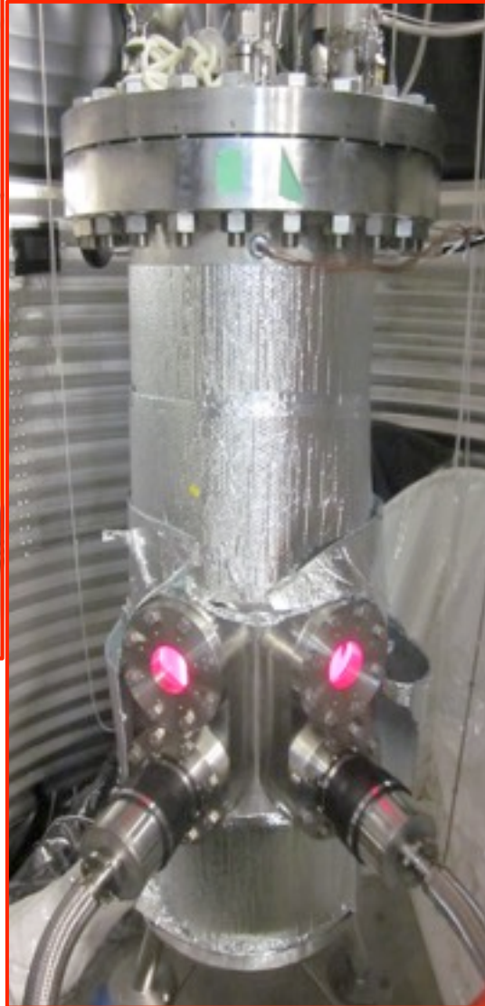
PICO-60 Pressure vessel inside the water tank at Snolab
