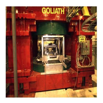
gap: height = 1050 mm diam. 2000 mm  $B_{MAX}$  = 1.5 Tesla
