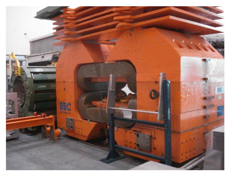
gap: height = 500 mm width = 1530 mm depth = 500 mm  $B_{max}$  = 1.65 Tesla
