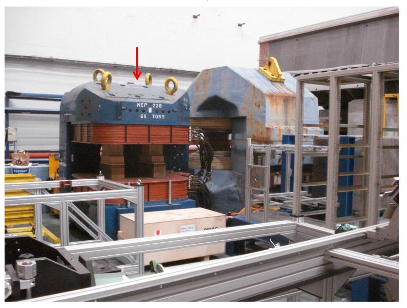
gap: height = 500 mm width = 1000 mm depth = 1000 mm  $B_{max}$  = 1.4 Tesla
