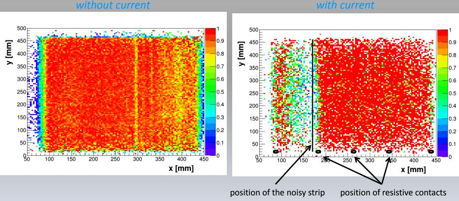
⇒ resistive ladders seem to spread the current around the resistive noisy strip
