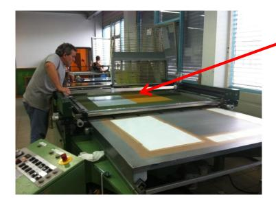
Semi automatic machine Printing area 1.5m x 0.9m
