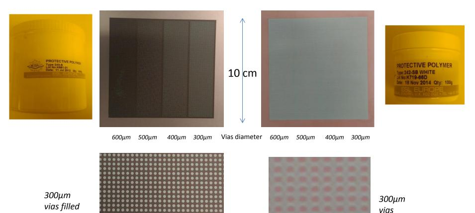
With this test We have seen that it's possible to process small pitches
