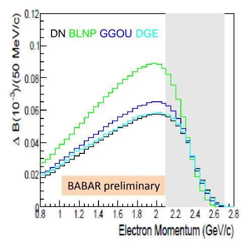
the results depend on the predicted shape of lepton spectrum for B→X<sub>u</sub>ev decays
