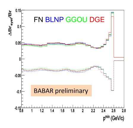
ΔB <sub>syst</sub> - systematic uncertainty for branching fraction in range p<sup>min</sup>-2.6GeV/c
