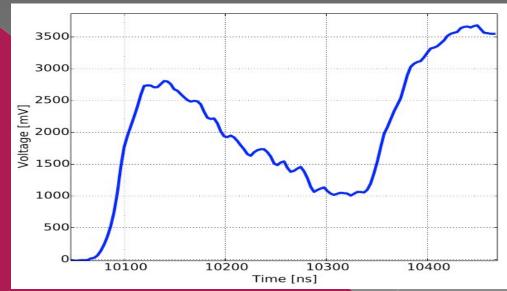
Simulated double pulse waveform from a  $v_{\scriptscriptstyle T}$  CC interaction
