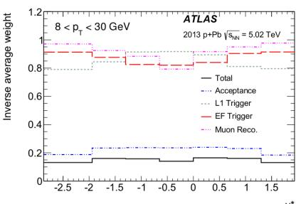
**L1 Trigger**: Measured with respect to Minimum Bias events
