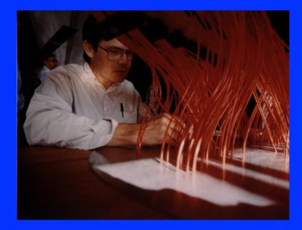
Fiber-fed spectrograph : 7 deg<sup>2</sup> field-of-view.
