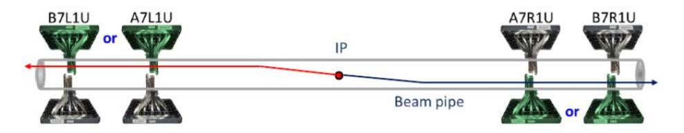
The ALFA detector is at 240m from the IP, the detector was placed at ~5mm from the beam, 800k elastic events were recorded.
