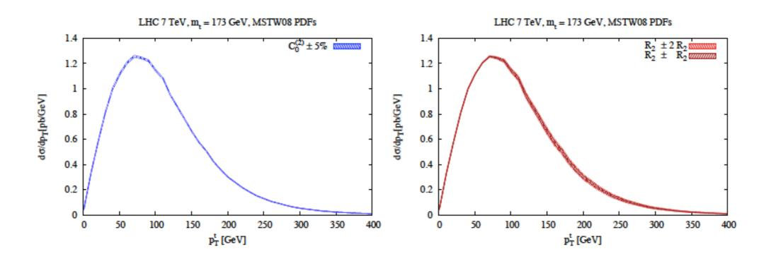
Left: The coefficient  $C_0^{(2)}$  (scale ind. contribution in  $D_{ij}^{(0)}$ ) is varied within its 5% while  $R_2$  is kept fixed. Right: here the coefficient  $R_2$  is varied by adding and subtracting  $2R_2$  while  $C_0^{(2)}$  is kept fixed.
