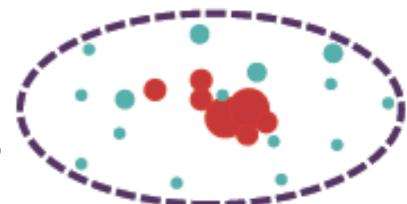
1. **Fat jet:** large distance parameter to pick up all the radiation from the original decay
