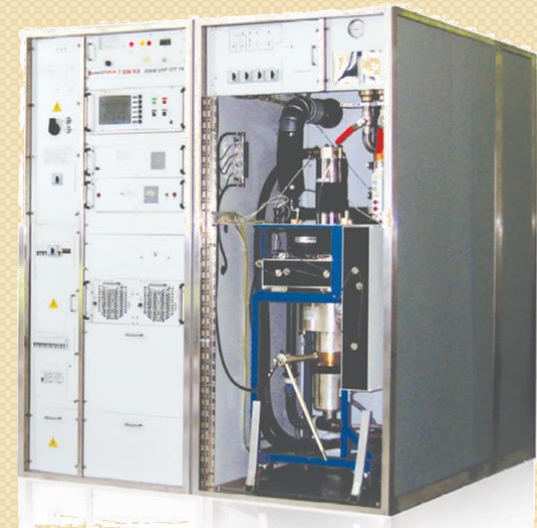
New CERN 802 MHz, 60 kW CW IOT TX 9 units received & tested
