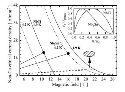
This is the graph of the critical values of flux density and current density shown on slide for NbTi and Nb<sub>3</sub>Sb at 4.2 and 1.9 K, as shown on slide 78.
