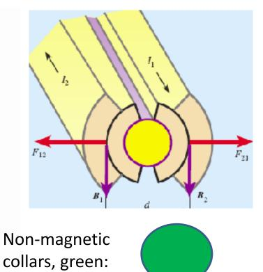
restrain bursting forces of 2.10<sup>6</sup> N/m.
